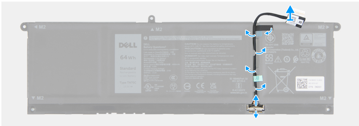
Figure 35. Removing the battery cable
