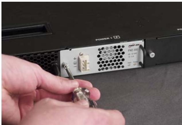
9. Connect the terminal block into the DC power supply.
