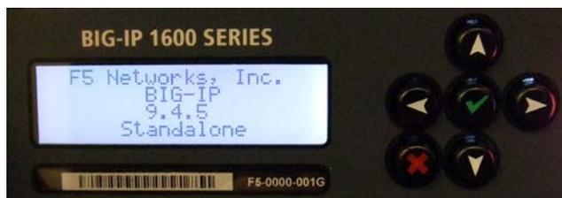
Figure 3: The LCD panel and control buttons
