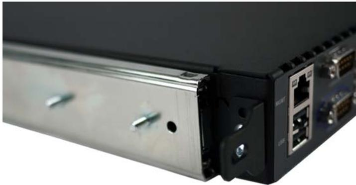
5. Attach the front mounting brackets to the outer rails, and then slide the front mounting brackets up to the rail locks.
