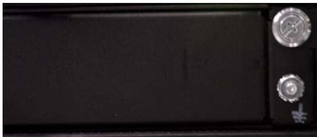
Figure 4: Chassis ground lug
