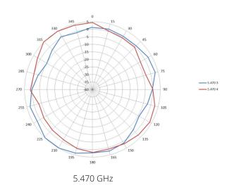
Elevation plane (side view, 0 degrees angle)
