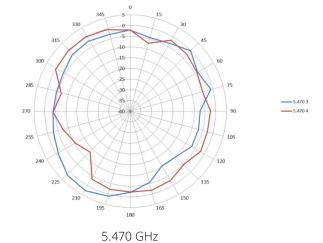
Horizontal or azimuth plane (top view), 30 degrees downtilt
