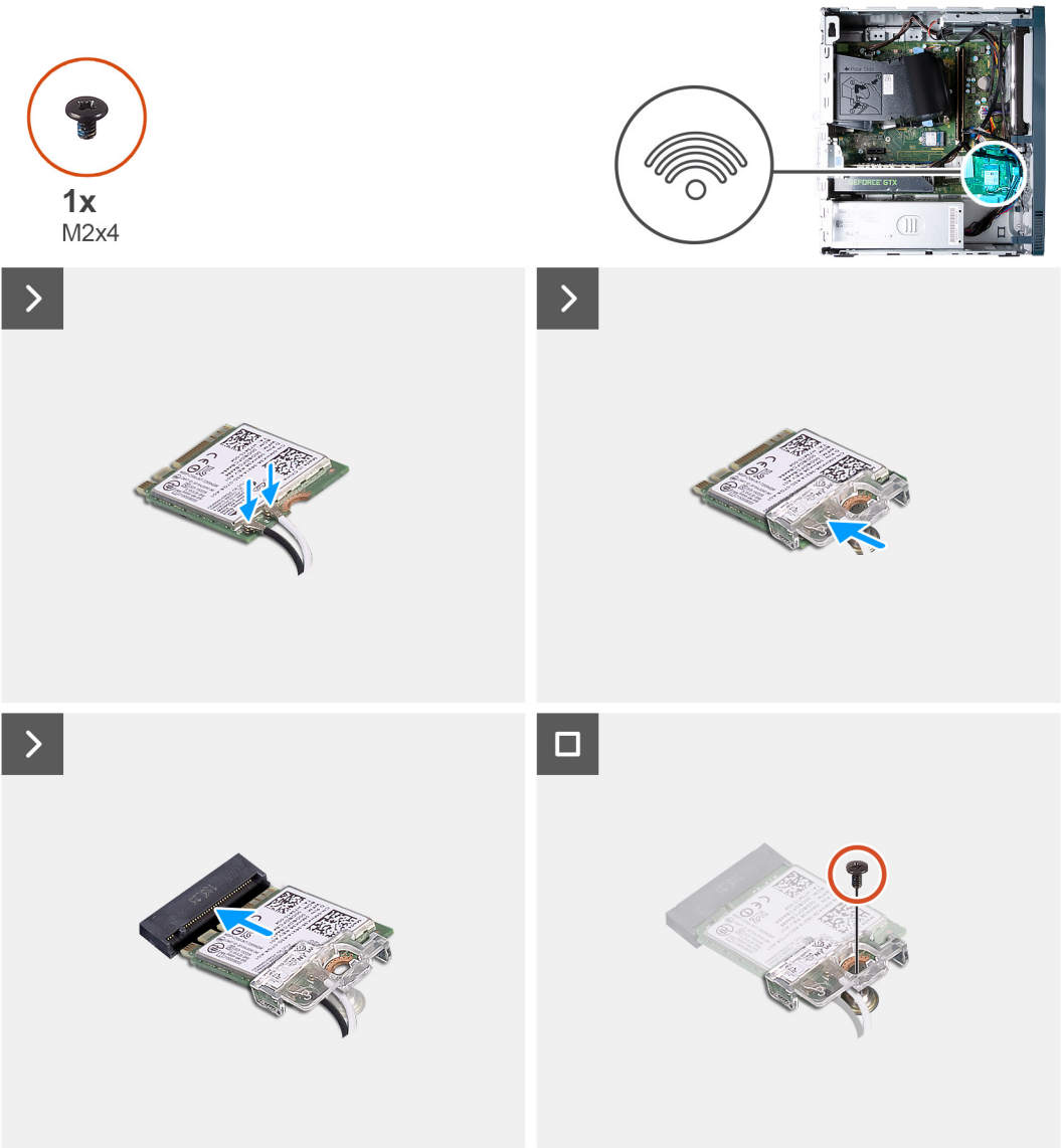
Figure 21. Installing the wireless card
