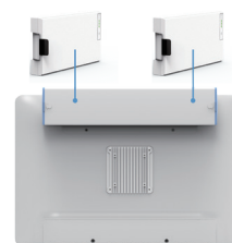
Battery module contains 2 x battery packs
