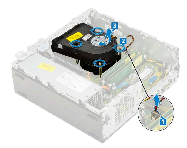
(i) NOTE: Loosen the screws in a sequential order (1,2,3,4) as mentioned on the system board.
