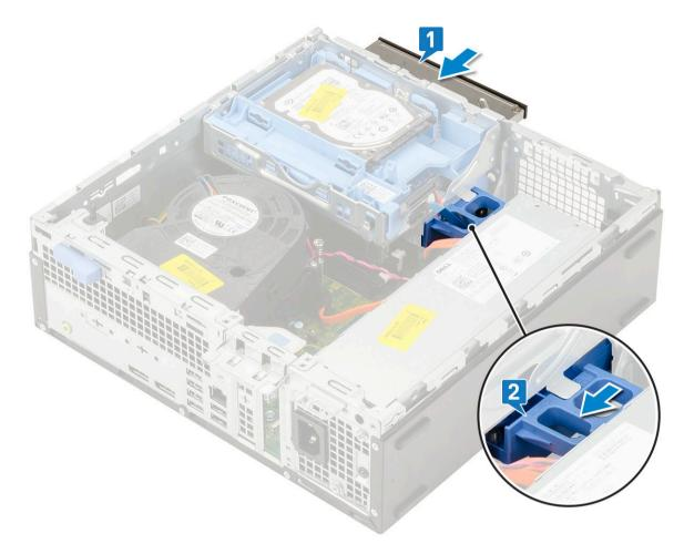
Lift the hard drive and optical module [1], connect the optical drive data cable and power cable to the connectors on the optical drive [2, 3].
