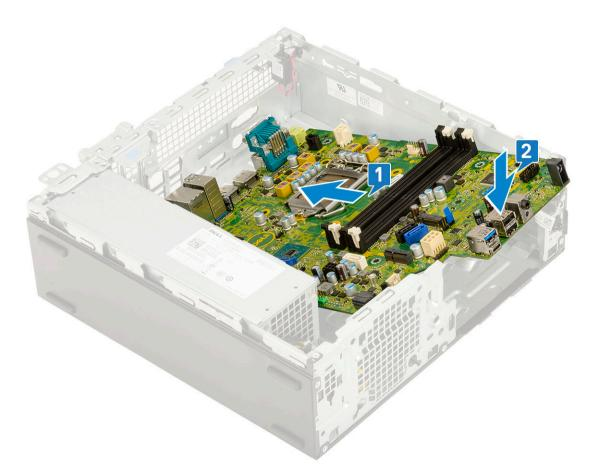
3 Replace the single screw used as a mounting point for M.2 SSD drive, the standoff single (#6-32) screw and the 5 screws that secure the system board to the system [1, 2, 3].
